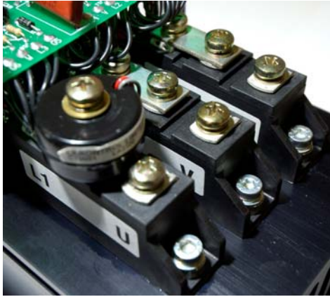
Showing the position of the bus-bar, linking on the supply inputs, (L1, L2 and L3) side of the thyristor Paks on units of 5.5kW through 37kW.
